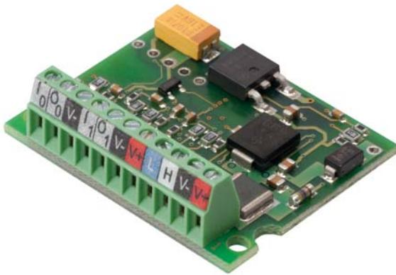
This **busstop** <sup>®</sup> station provides a connection for two input and two output points. All inputs and outputs are powered by DeviceNet™. This is ideal for small systems that don't require auxiliary power.
